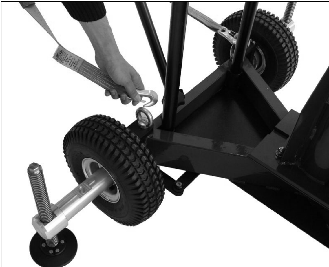
1.1.a - Snap hook at eyebolt on dolly
