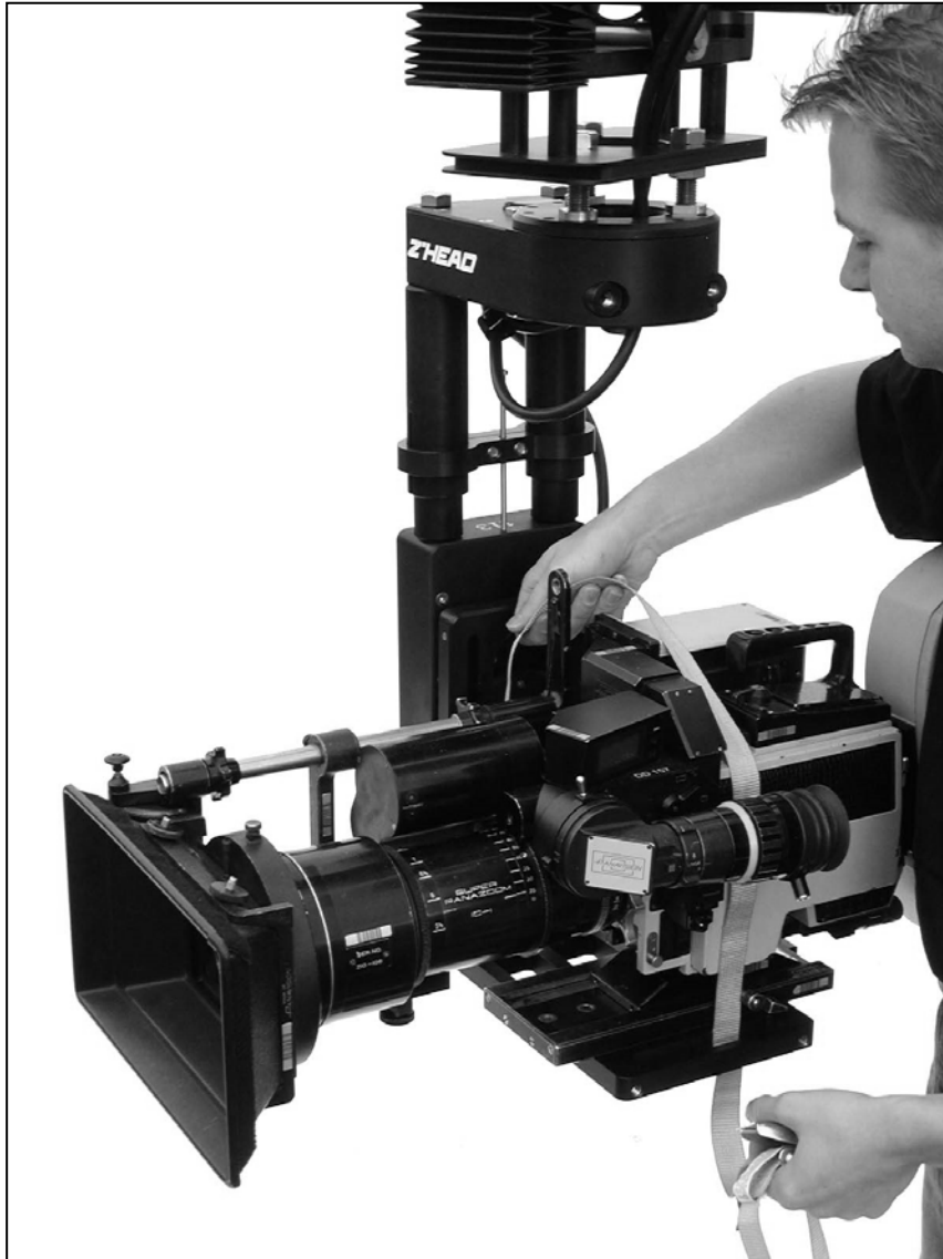
2.8.2.b - Securing the camera with a strap
