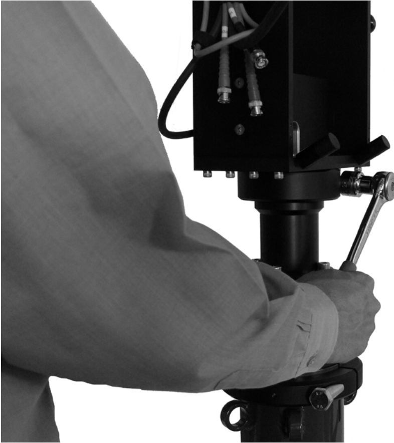
2.3.5. - Locking horizontal brake
