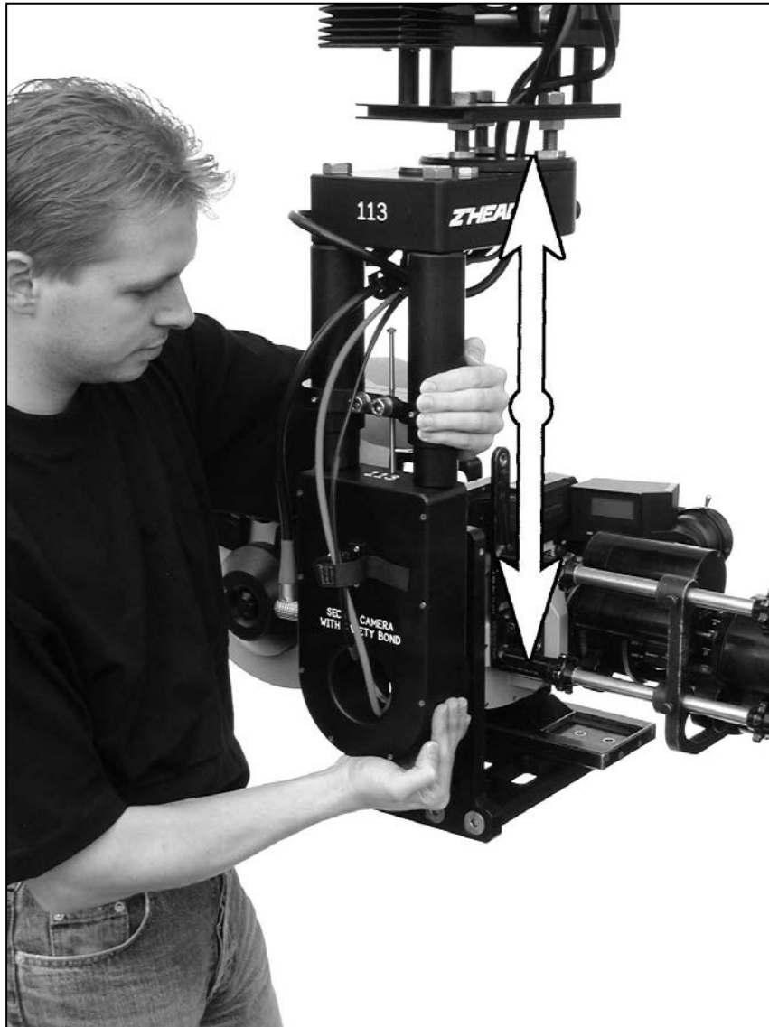
2.8.4. – Moving raiser up and down
