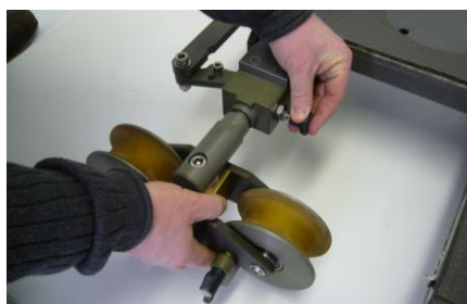
Removing the track wheel
