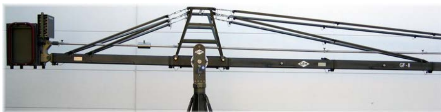
Double Rigging System
