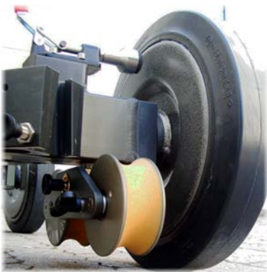
Wheel brake on Base Dolly
