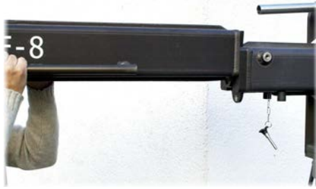
Mounting an extension arm
