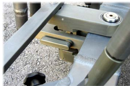
Switch lever (here in middle position)
