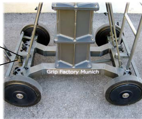
Dolly Double Ended Connected Steering
